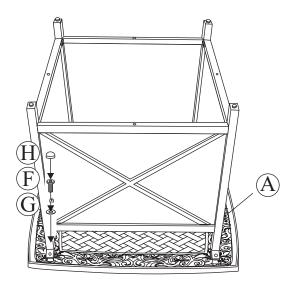
Attach the bottom panel with umbrella base pole to the table leg(B) & side panel(C) by using the bolts and washers as shown in **Fig.4**. Guide these bolts and washers through the holes in bottom panel, into the pre-drilled holes in the table leg (B) & side panel (C). **Hand tighten only.**
