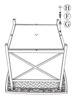
After adjusting any necessary alignment of legs, side panels, and bottom panel, use the hex bolt driver to tighten all bolts. **Note:** each bolt must be tightened a few revolutions at a time. In order to apply equal pressure to all bolt joints, we recommend working in a cross corner (X fashion). Repeat until all bolts are tight. **Do not over tighten**. Over tightening may strip bolts. Cover all bolts with covers.
